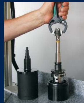
Using the handling pliers, slide the shrink ring over the tool holder
