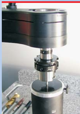
Heat the shrink fit chuck. As soon as the shrink fit chuck achieves shrink-out
