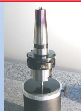
Place the shrink fit chuck on the pin.
