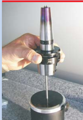
Determine the length up to the stop of the tool cutting edge.
