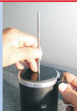
Adjust the length of the pin of the ejection device (up to the stop + approx. 2 cm)
