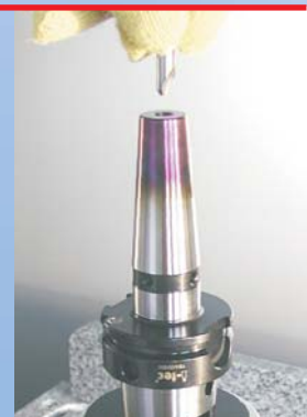
The broken cutter shank can then be removed easily.
