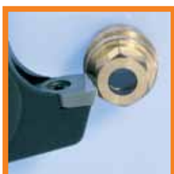
Polygon turning: Establishing of flats i.e. hex directly on lathe
